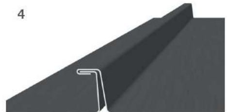
First turn completes angle standing seam joint
