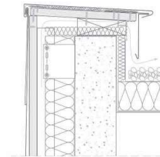
Rear vented capping (Rhomboid tile)
