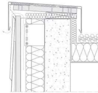
Front vented capping (square tile)
