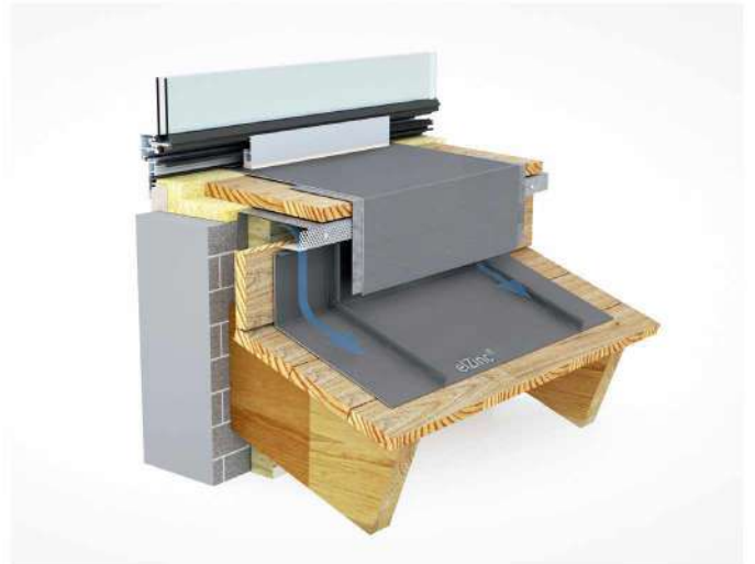
DLSS 6.1.01 – Vented abutment (under window).
