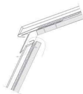
Vented transition mansard roof
