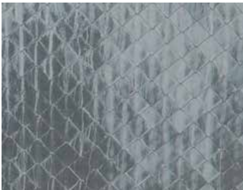
Staining caused by cleaning of adjacent brickwork by baking soda. These stains are difficult or impossible to remove without damaging the pre-weathered surface of Alkimi products, due to the chemical bonding of the contaminant to the surface. Depending on the aggressiveness of the cleaning products, also Rainbow and Advance finishes can be affected
