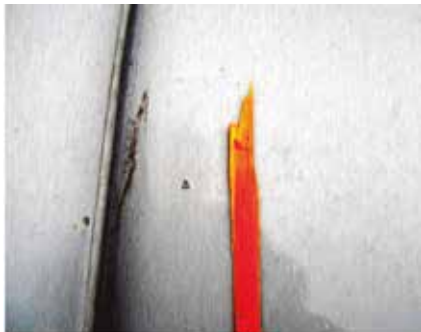
Wood chips and splinters absorb moisture, and can stay humid for enough time to mark the bright zinc surface. Care should also be taken with elZinc Alkim® , Rainbow and Advance.
