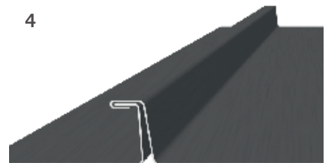
First turn completes angle standing seam joint
