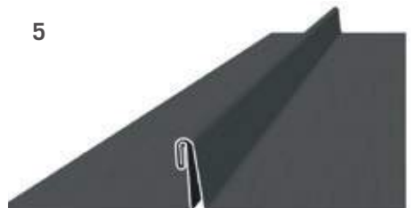
Double lock welt, second turn completes double lock standing seam joint
