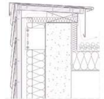
Rear vented capping (fish scale tile)
